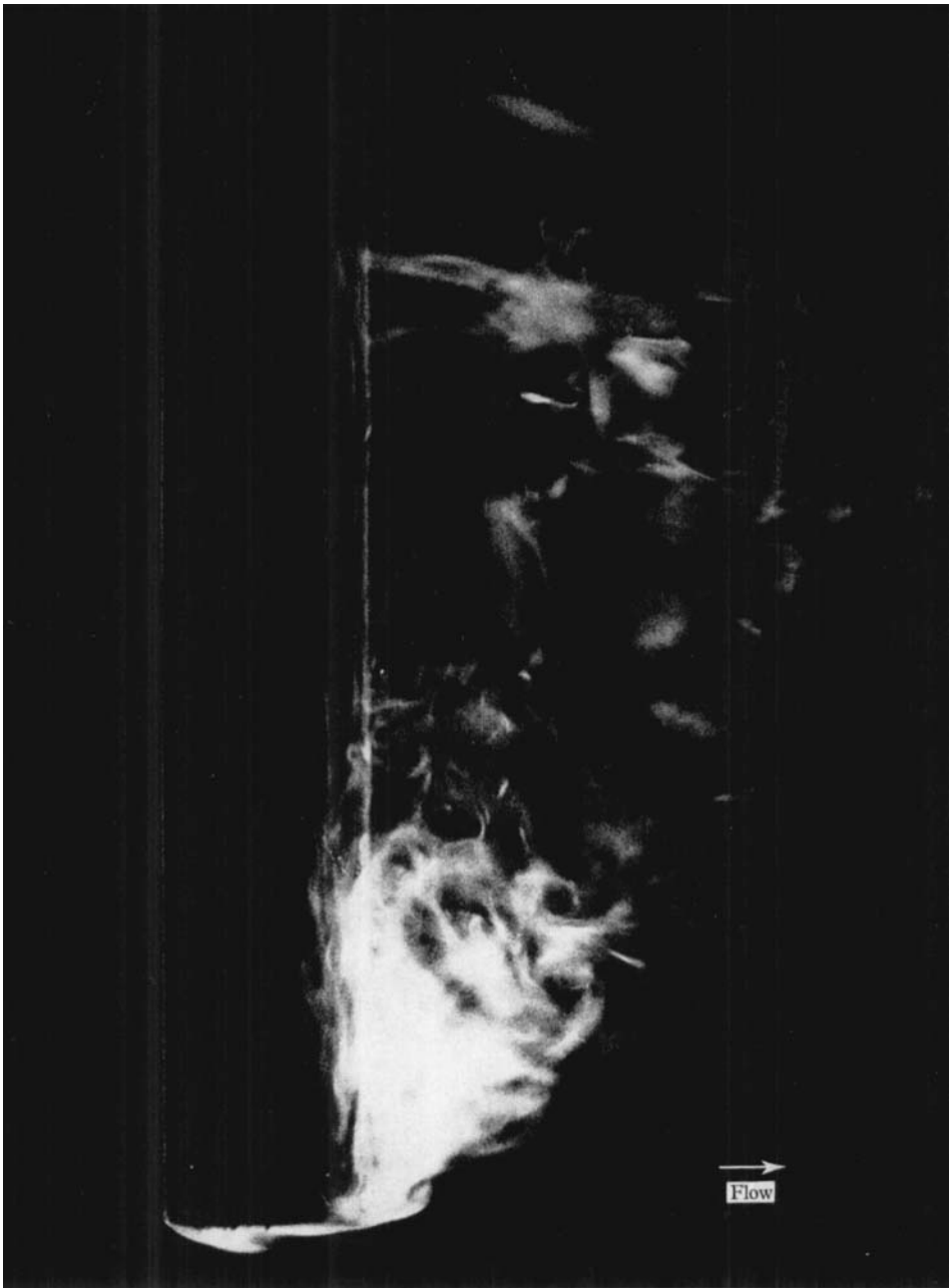
FIGURE 11. Illumination of the wake behind a circular cylinder. Flow is from left to right.
